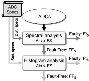
Figure 1. Classical ADC Test flow
