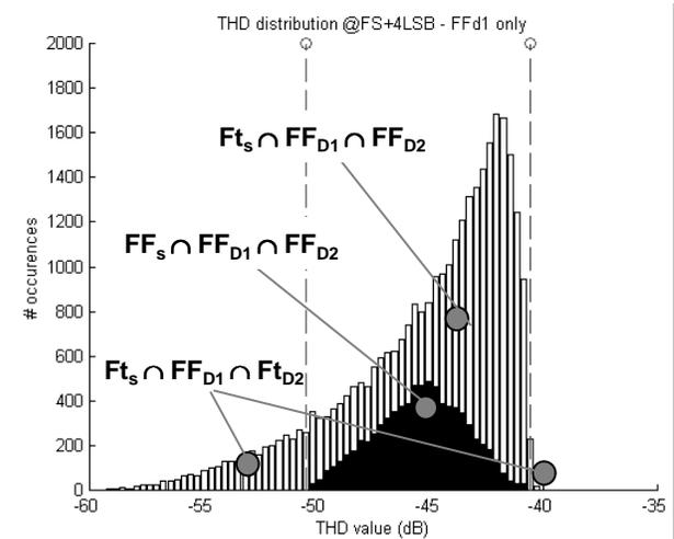
**Figure 6. Distribution of the measured dynamic values (with  $A_{in} > FS$ ) for each dynamic parameter (SINAD, SFDR & THD) over the population appreciated as fault-free by the classical FFT procedure ( $FF_{D1}$ )**
