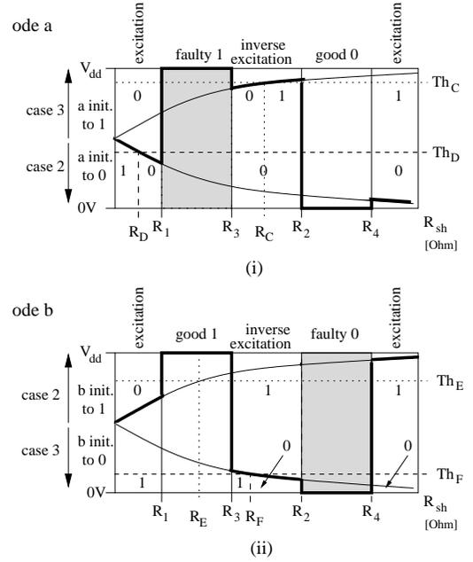
Figure 4: Voltage depending on bridge resistance  $R_{sh}$
