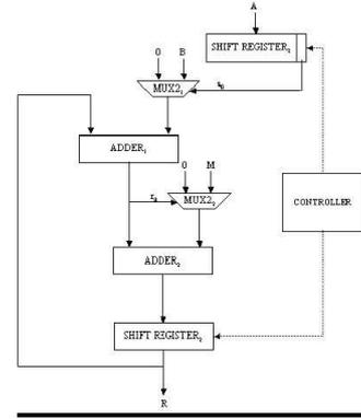
Figure 5 - Nedjah's [15] iterative modular multiplier
