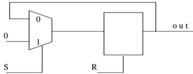
**Figure 1: Example of stuck at 0 FF**
