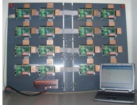
Figure 8 Array of 4x4 NPU multi board.
