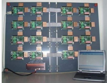
Figure 8 Array of 4x4 NPU multi board.
