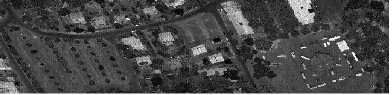
Figure 1: Amplitude image of the first echoes detected by the embedded real-time system, displayed in the sensor geometry.
