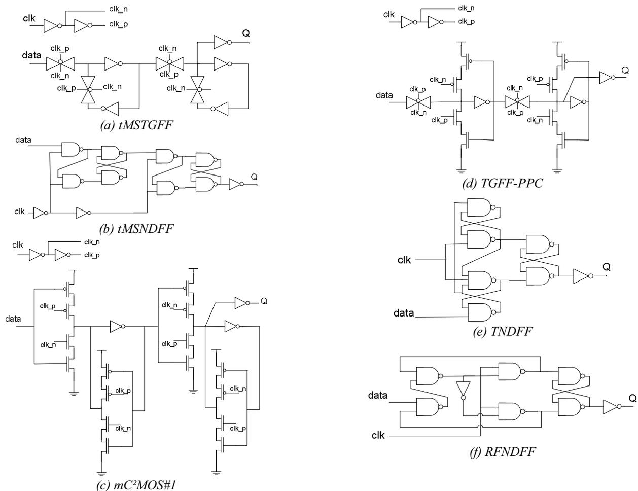
Fig. 1. Schematics of the FF chosen in the study. All are static flip-flops. (a) is the *Typical Master Slave FF based on transmission gates* (b) is the *Typical Master slave FF based on NAND gates* (c) is the *Modified C<sup>2</sup>MOS FF #1* (d) is the *PowerPC 603 FF/ TGFF* (e) is the *True NAND-based DFF* (f) is the *Race-Free NAND-based DFF*
