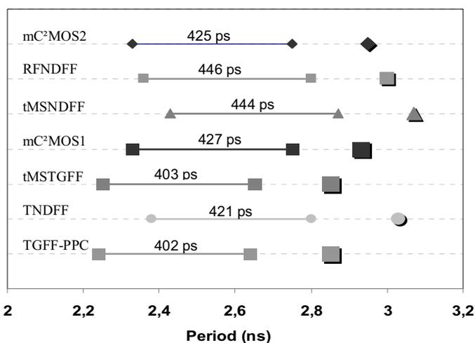
Fig. 3 : This graph represents the period range corresponding to a setup time violation probability between 90% and 10%. The single points refer to a violation probability of 0.5%.
