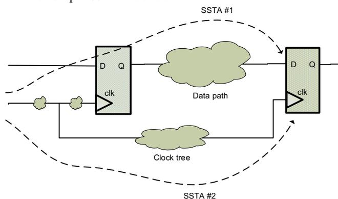
Fig. 2 : Two SSTA are performed : one on the data path, the other on the clock path. The information obtained allows to calculate the setup/hold time violation probability on the second D-flip-flop.
