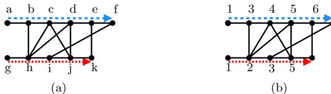
Fig. 1. An instance (G, R, P) of min-DAWN-path containing 2 requests r_1 = (a, f) , r_2 = (g, k) , P(r_1) = (a, b, c, d, e, f) and P(r_2) = (g, h, i, j, k) (sub-fig. a). A valid and conflict-free date assignment and within a minimum number of slots (sub-fig. b).
