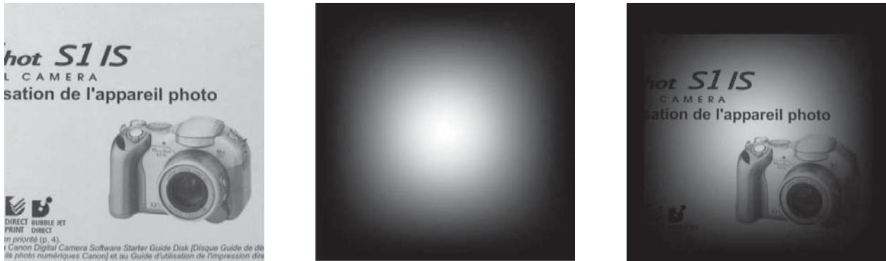
FIG. 4 – (a)-Original image (left), (b)-Imaging system response (center) (c)-Obtained image (right)
