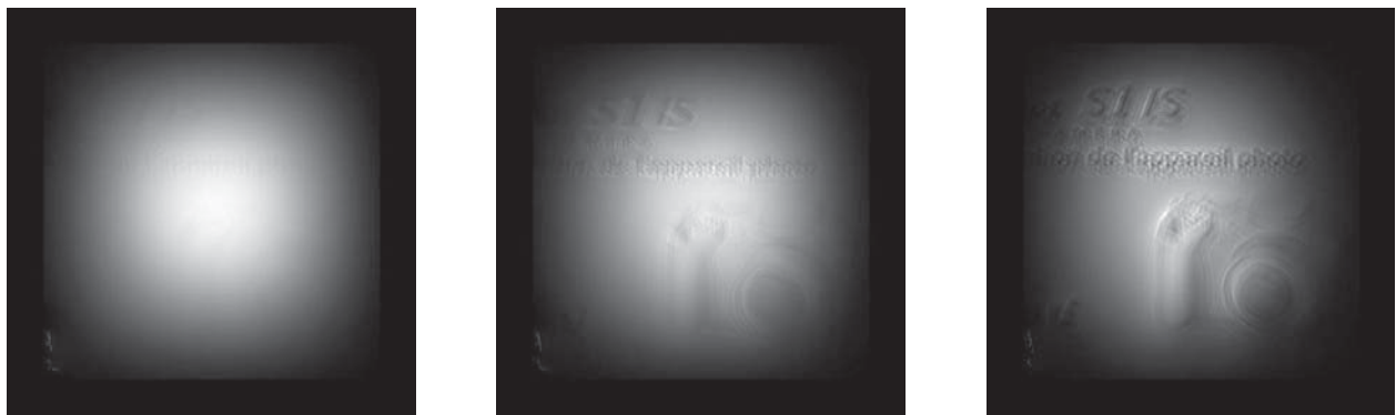
FIG. 18 – Ghost effects on resulting image V(x, y) using synthetic images : errors effects on the translation vectors (slight errors (left), mean errors (center), large errors (right))
