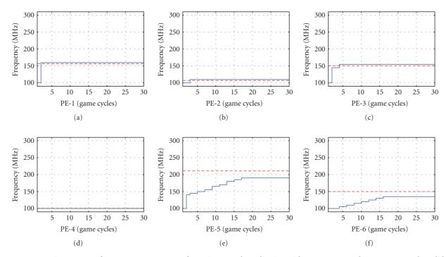
FIGURE 8: Dynamic response of a  $3 \times 2$  processor array for a given 6-task application with  $w_{syn} = 0.75$  and  $w_{temp} = 0.25$ . The solid line shows the evolution of the chosen frequency for each PE. The NE is defined by  $f_1 = 160$ ,  $f_2 = 110$ ,  $f_3 = 155$ ,  $f_4 = 100$ ,  $f_5 = 190$ , and  $f_6 = 135$  MHz. The dashed line is the reference solution calculated by Matlab:  $f_1 = 156$ ,  $f_2 = 107$ ,  $f_3 = 149$ ,  $f_4 = 100$ ,  $f_5 = 210$ , and  $f_6 = 149$  MHz.
