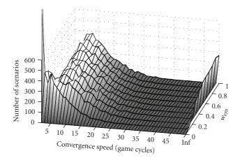
FIGURE 5: Weights exploration for a  $5\times5$ -processor array. The *x*-axis represents the number of scenarios over 50 000 simulations. The *y*-axis shows the convergence speed in game cycles, while the *z*-axis explores the weight of the synchronization metric  $w_{syn}$ . The inflabel on the *y*-axis denotes those cases which do not converge.
