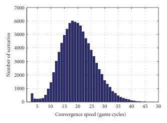
FIGURE 3: Convergence speed distribution for a 100-processor platform with  $w_{syn} = 1$  and  $w_{temp} = 0$ : the average speed is 18 game cycles.
