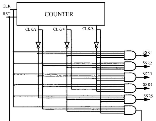
Fig. 2. The counter/decoder.
