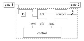
Fig. 2. Activity counter (dashed block) inserted at the output of gate 1
