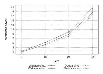
Fig. 6. Power estimation results compared to Spice simulations
