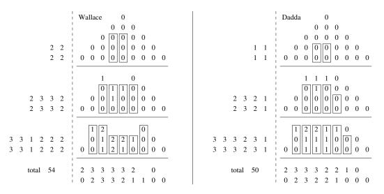
Fig. 5. Glitching activity estimation for 5-bit partial products trees using degree-0 polynomials and all coefficients equal to 1
