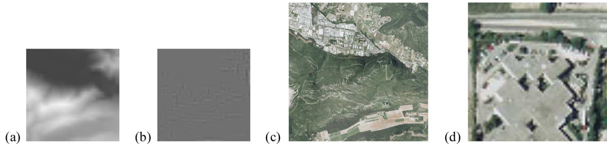
Fig. 9. Reconstruction of the images from the approximation image at Level 1: (a) extracted altitude, (b) difference image between the original altitude and the extracted one, (c) texture, and (d) magnified part of texture corresponding to Fig. 7(c).
