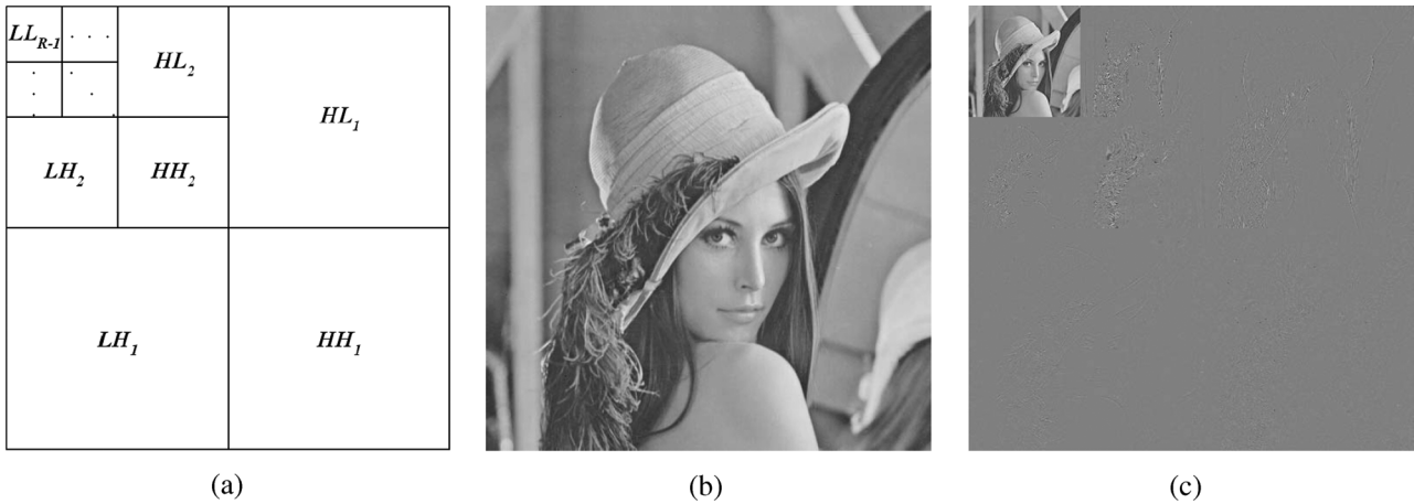
Fig. 2. DWT: (a) Subband structure, (b) Lena, and (c) Lena at level 2 DWT decomposition.
