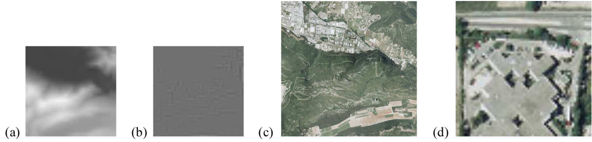
Fig. 9. Reconstruction of the images from the approximation image at Level 1: (a) extracted altitude, (b) difference image between the original altitude and the extracted one, (c) texture, and (d) magnified part of texture corresponding to Fig. 7(c).
