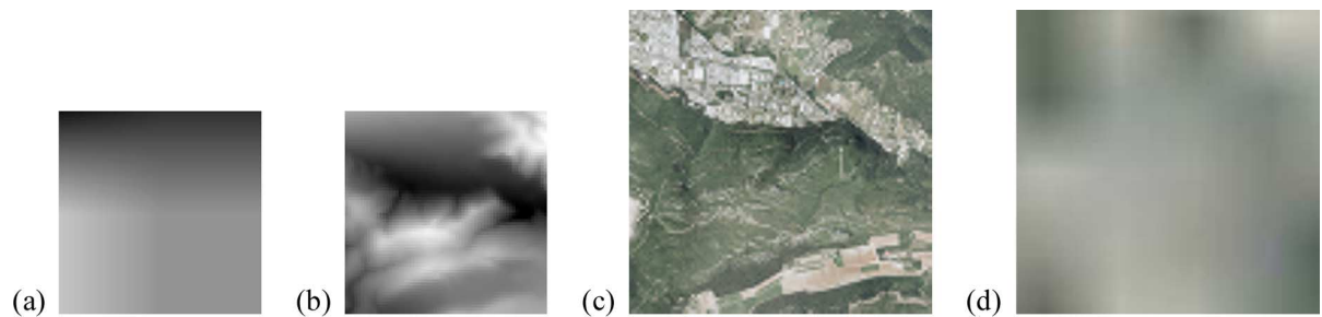
Fig. 12. Reconstruction of the images from the approximation image at Level 5: (a) extracted altitude, (b) difference image between the original altitude and the extracted one, (c) texture, and (d) magnified part of texture corresponding to Fig. 7(c).
