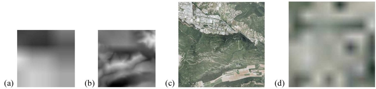
Fig. 11. Reconstruction of the images from the approximation image at Level 4: (a) extracted altitude, (b) difference image between the original altitude and the extracted one, (c) texture, and (d) magnified part of texture corresponding to Fig. 7(c).
