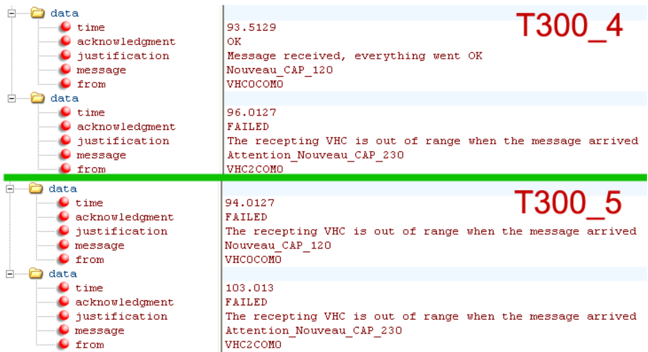
Fig. 14. Attenuation error: the level of the propagated messages is too low to be understood by the receiving AUVs
