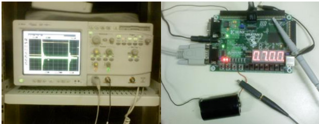
Fig. 7 DPA/CPA Measurement setup.
