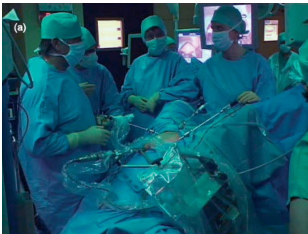
Figure 6. First in vivo procedure. (a) Main structure mounted on the lateral rail of the table and covered by a sterile plastic bag. (b) The compactness of the robot allows all the team members to stand next to the table and work normally without being bothered by its presence
