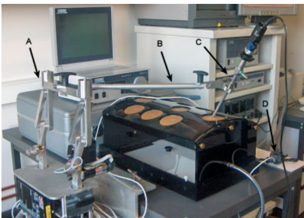
Figure 4. Prototype of the device on the pelvitrainer, composed of main active manipulator A, simplified arm B, manual laparoscope clamp C and miniature joystick D mounted on a surgical instrument
