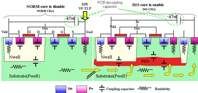
Fig. 1. Comparison between NORM and ISO core architectures
