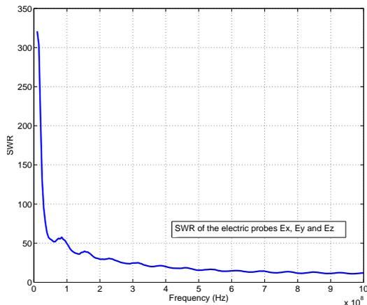
Fig. 9. SWR of the electric probe
