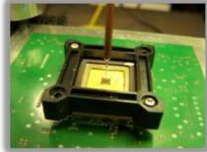
Fig. 3. Photograph of an electric field ( $E_z$ ) injection
