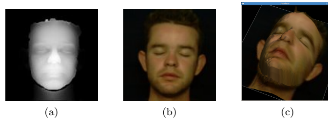
Fig. 2: Original data: a) 120 \times 120 depth map (2.5D), b) The corresponding 120 \times 120 2D face image, c) A 3D face view obtained from (a) and (b)
