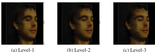
Fig. 5: 3D visualization corresponding to Fig. 2 realized through the overlaying of level- l approximate texture on the extracted level- (l-1) approximate depth map.
