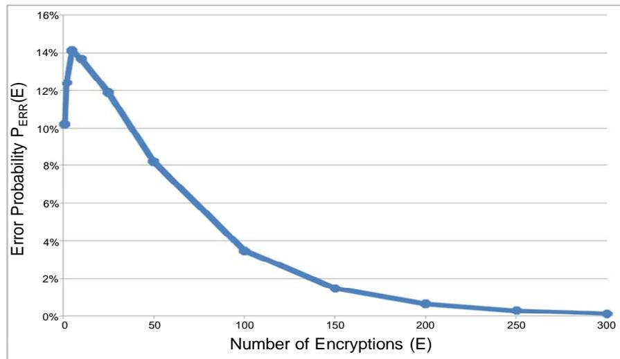
**Figure 7: Error probability w.r.t. the number of encryptions**
