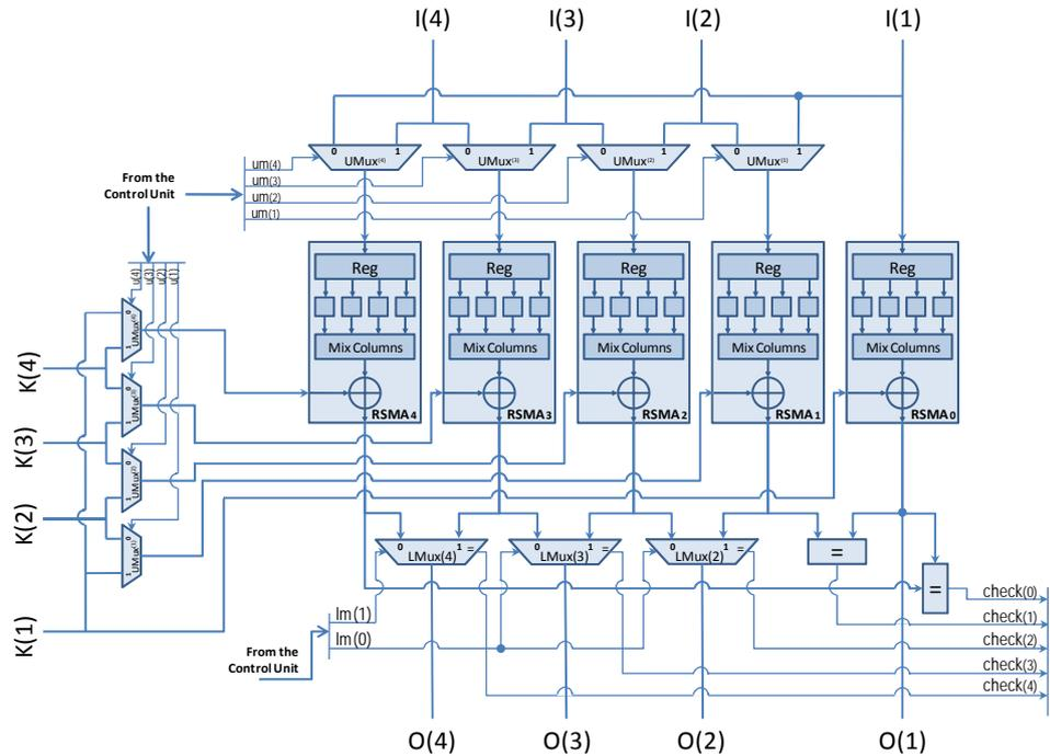
**Figure 4: AES Architecture with RSMA duplication and comparison**
