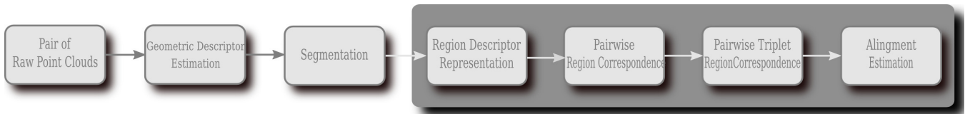
Fig. 1: Region-based global registration algorithm pipeline. This paper contributes the outlined stages of the global registration pipeline.
