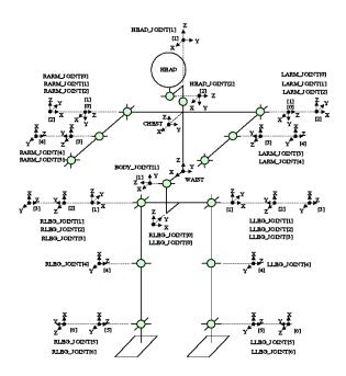
Fig. 2. Denavit-Hartenberg parameters definition coordinate of the HOAP-3 Robot
