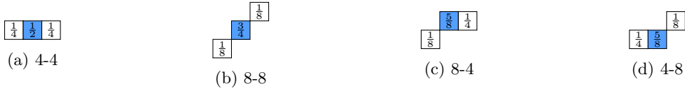
Fig. 3: There are only four equivalence classes appearing on an 8-connected line in the first octant.
