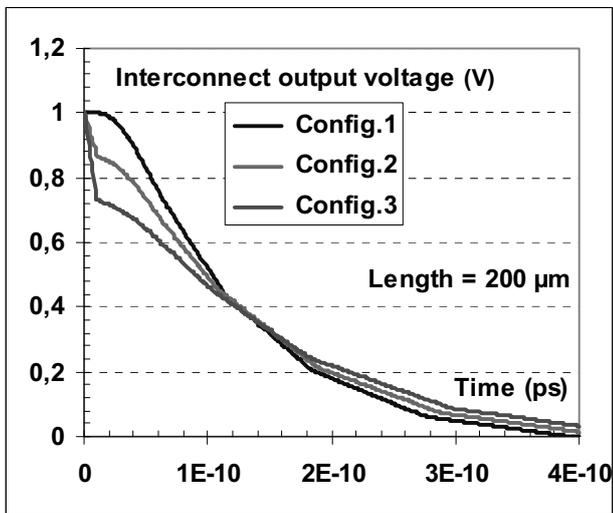
Fig. 3: Inner interconnect output voltage for different propagation configurations by using an RC model for the interconnects.
