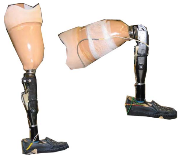
Fig. 2. The constructed prototype of the knee prosthesis.
