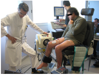
Fig. 5. The experimental setup: the torques around knee joint are measured in isometric condition through the Biodex system.
