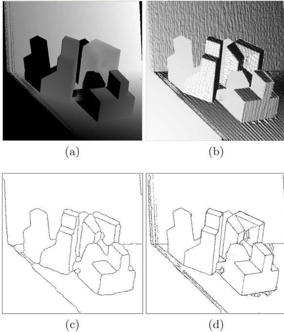
**Fig. 2.** The impact of the alteration strength on the segmentation results: (a) Range image (abw.test.8); (b) Rendered range image; (c) Segmentation results with  $\xi_{min} = \xi_{max} = 4$  at  $t=2500$ ; (d) Segmentation results with  $\xi_{min} = 0.3$  and  $\xi_{max} = 5$  at  $t=13000$
