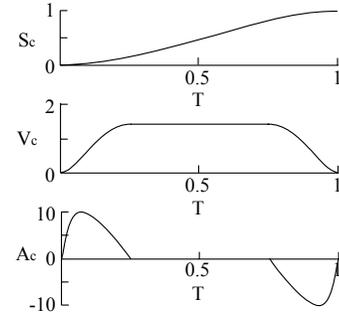
Fig. 13. Cam curve.
