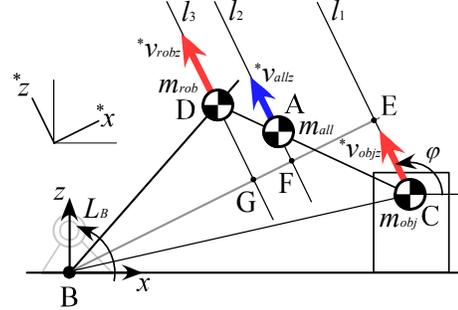
Fig. 11. Position and velocity of CoM when lifting.
