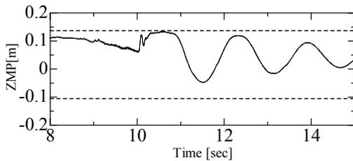
Fig. 17. Experimental result of the ZMP position.
