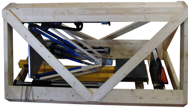
Figure 20: Prototype of MoM3 with a wooden frame and arms
