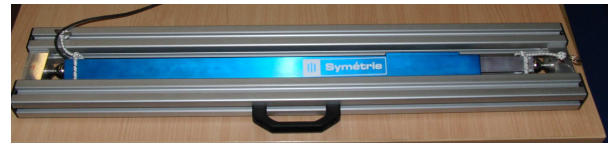
(b) Gough platform strut in the calibration artefact. This equipment has been designed following our specifications by Symétrie Co. Nîmes, France.
