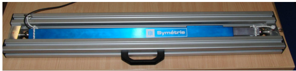
(b) Gough platform strut in the calibration artefact. This equipment has been designed following our specifications by Symétrie Co. Nîmes, France.
