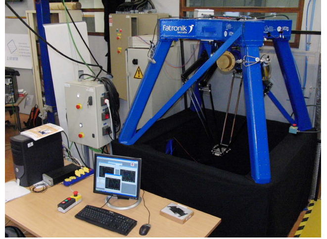
Fig. 2. Par2 parallel manipulator experimental setup
