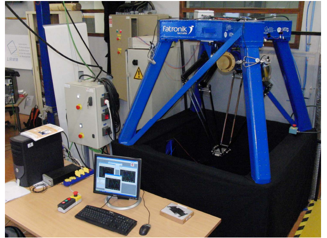
Fig. 2. Par2 parallel manipulator experimental setup
