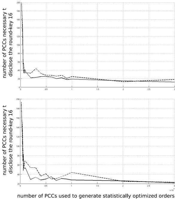
Fig. 2. evolution of the number of  $PCCs$  necessary to disclose the key functions on the number of  $PCCs$  used to generate the *statistically optimized orders*. DPA (upper) and CPA (lower). Solid lines correspond to method 1 whereas dashed lines to method 2
