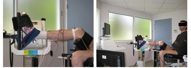
Fig. 2. Electrodes configuration (left) and experimental set-up (right).
