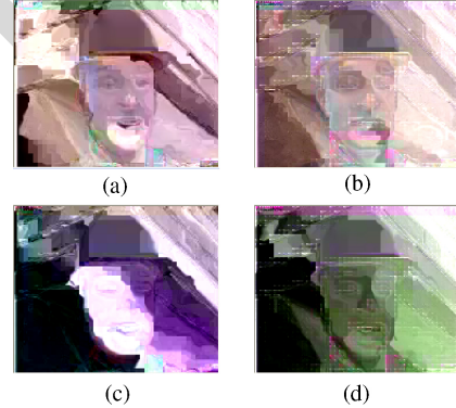
Fig. 14. Attack in the selectively encrypted image by removing the encrypted data. (a) SE-CAVLC encrypted image \{Y, U, V\} = \{10.01, 26.86, 25.24\} dB. (b) SE-CAVLC attacked image \{Y, U, V\} = \{8.87, 27.3, 26.3\} dB. (c) SE-CABAC encrypted image \{Y, U, V\} = \{8.20, 17.95, 24.53\} dB. (d) SE-CABAC attacked image \{Y, U, V\} = \{7.72, 28.6, 24.6\} dB.
