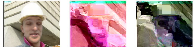
Fig. 13. Key sensitivity test for encrypted frame #1 of Foreman video sequence for QP value 18. Encrypted frames are decrypted and decoded with (a) original key, (b) 1-bit different key (SE-CAVLC), and (c) 1-bit different key (SE-CABAC).
