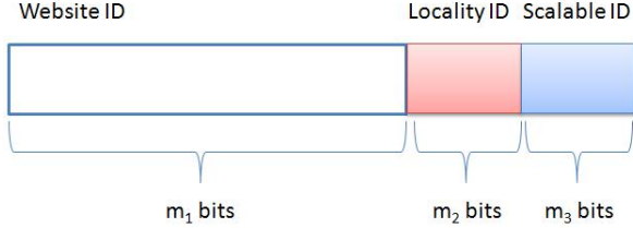
Figure 5: Peer ID structure in D-ring of PetalUp-CDN.
