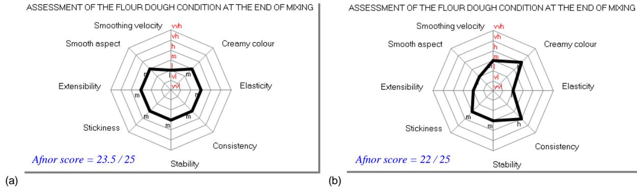
Figure 5: Examples of the KBS outputs: predictions of dough state at the end of texturing, starting from a standard consistency at the end of first mixing ( $350 \leq w \leq 450$  UB), a standard target temperature ( $22 \leq x \leq 25$  °C), an average difference of velocity  $y$  and a heat dissipation  $z$  (a) medium and (b) low. Scale ranges from vvh (very excessive) to vvl (very insufficient).
