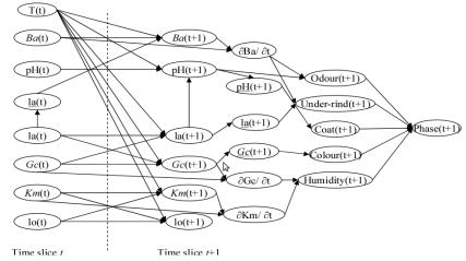
Figure 6: Dynamic Bayesian network representing the coupled dynamics of micro-organism growth with their substrate consumptions influenced by temperature and involving the sensory changes of cheese during the ripening process.
