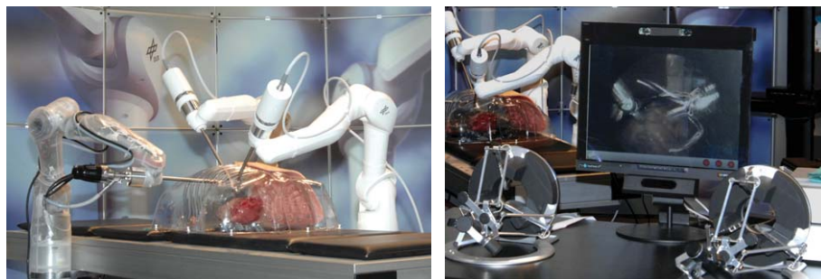
Fig. 1. The MiroSurge System: Slave side (left) and master side (right).
