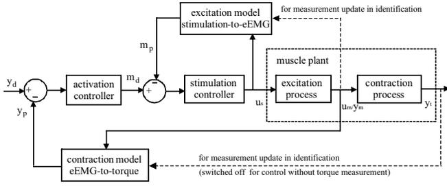
Fig. 2. Diagram illustrating the dual predictive control using biofeedback. The control signal obtained from activation controller is used as desired reference of stimulation controller. In each controller, nonlinear generalized predictive control algorithm was applied based on a PHM model. The torque measurement  $y_i$  and eEMG measurement  $u_m/y_m$  were only used for model identification as shown in dashed lines.
