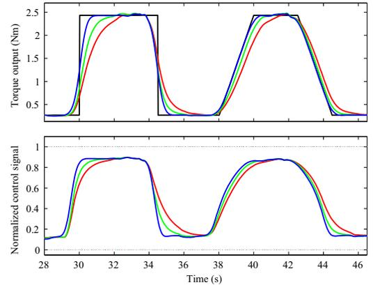
Fig. 7. Comparison of tracking performance with different types of torque trajectory. Different weighting coefficients were also tested. The weighting coefficient of input was chosen as DPC1 (red,  $\delta_1 = 0.1$ ,  $\delta_2 = 20$ ), DPC2 (green,  $\delta_1 = 0.5$ ,  $\delta_2 = 5$ ) and DPC3 (blue,  $\delta_1 = 20$ ,  $\delta_2 = 2$ ).
