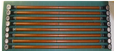
Figure 8. Par2's arms equipped with the piezo patches
