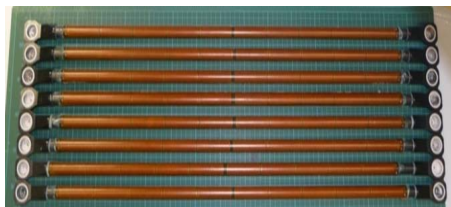
Figure 8. Par2's arms equipped with the piezo patches
