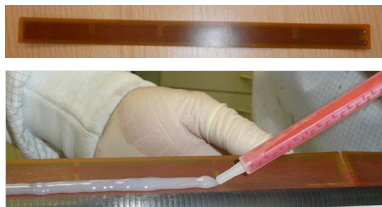
Figure 7. Piezo patch (top) and its fixation process (bottom)
