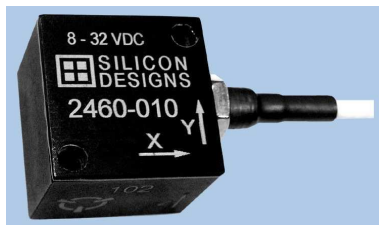
Fig. 19. External accelerometer used in the experiments*
