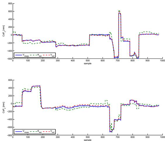
Fig. 2. Estimation of CoM position for the validation data set (Sb01). The plots indicate CoP position measured with the force plate ( $V_{meas}$ ), the estimated CoM  $K_{est}$  and  $V_{est}$  from the SESC models established with Kinect and Vicon measurements respectively.
