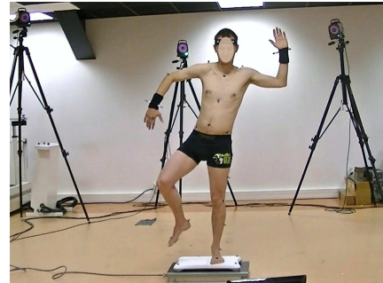
Fig. 1. Experimental setup for parallel measurement of Kinect-Wii board and Vicon-force plate.
