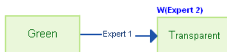
Figure 3.20: Green is the chosen value even though Transparent is wanted by Expert 2, because Transparent has an incoming arrow, which means that there is another value more preferred by a stakeholder.
