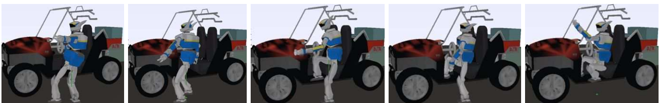
Fig. 5. Main snapshots from multi-contact planning of HRP-2 ingress in a car (model suggested by DARPA). From left to right: right after the initial posture, few steps with a support on the steering wheel (that is not yet mobile in the simulation); a support found by the right hand on the car's seat; unsuccessful ingress trial with the left foot; withdrawing left foot tree and engage ingress with the right foot; and finally a successful ingress with other few steps in the car. Note that no other knowledge except initial and final position is provided: the car model and its possible contact support areas is given together with that of the HRP-2. This scenario was also planned with the three robots and outcome a different contact supports for the three of them.
